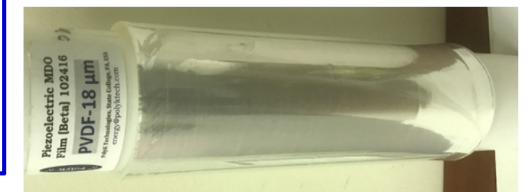
Machine-Direction Orientation MDO for Piezoelectric Film: 600 mm width and 2-20 m/min
